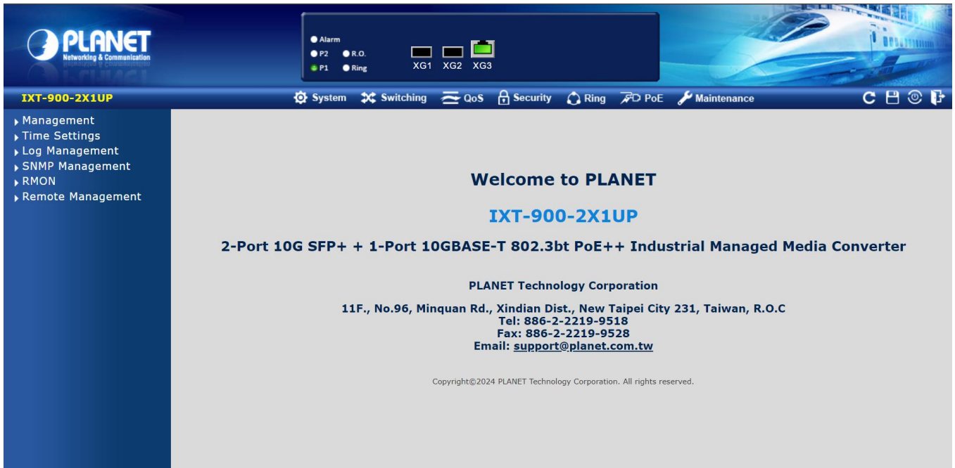
Figure 3-7: Web Main Screen of Industrial 10G Managed Media Converter
